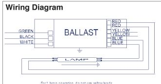
The wiring diagram that appears above is for the lamp type denoted by the asterisk (\*)
