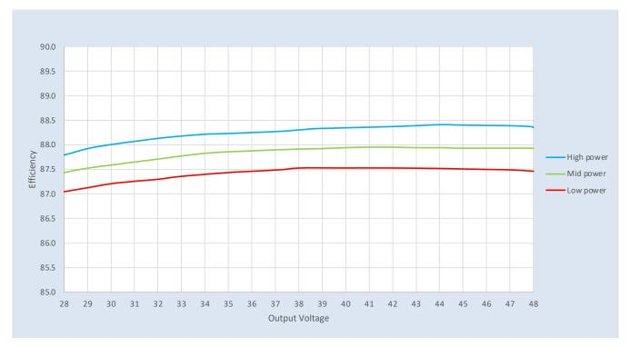
Efficiency Vs. Output Voltage at 277Vac Input
