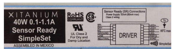
Figure 13. Product label indicating T_c point of driver in T-can
