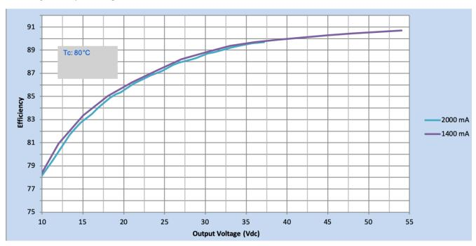
75W 0.1-2A 54V 0-10V INT (1% dim) with SimpleSet and auxiliary power supply selectable
