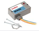
Emergency Lighting Control Device Supports lighting loads up to 10A Operates directly from fire alarm panel 24VDC
