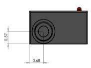
Nipple fitting for 1/2" trade size knockout (0.875" diameter hole)
