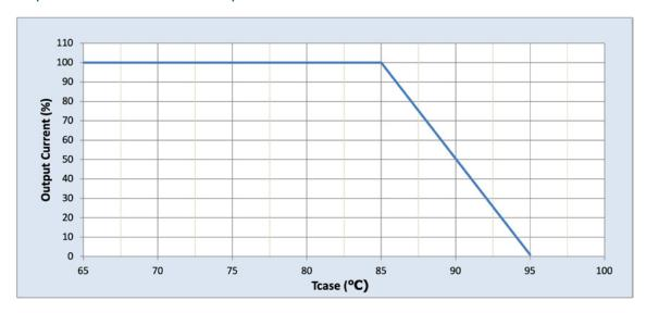
Note: There is  $\pm 5^{\circ}$ C tolerance on the driver case temperature
