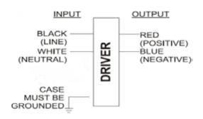
Input and output use lead- wires.
