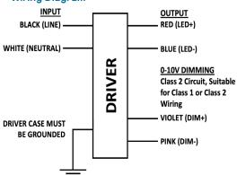
Input and output use lead- wires.
