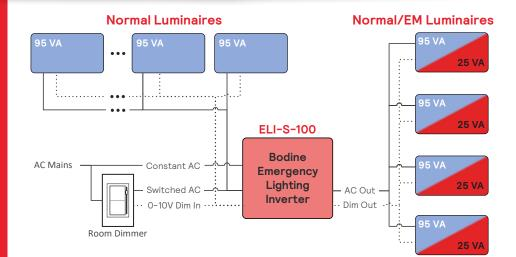
Above, while in the AC mode, the Normal/EM Luminaires have a total max power of 380 VA (4 x 95 VA). When in the emergency mode, Auto-Dim, using the DIM Out signal, reduces the power needs of each luminaire to only 25 VA each, 100 VA total.
