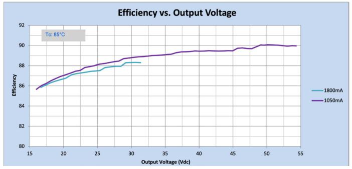
Efficiency Vs. Output Voltage at 277Vac
