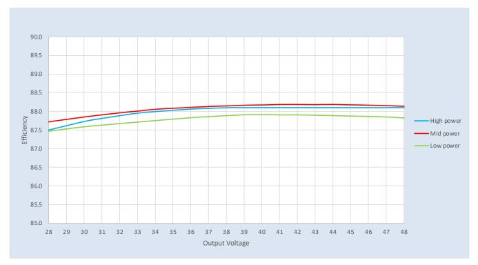
Efficiency Vs. Output Voltage at 277Vac Input
