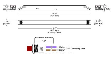
An illuminated test switch/charging indicator light is provided.
