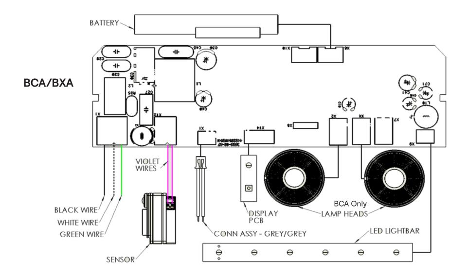
**NOTE 1:** For short-term testing of the emergency function, the battery must be charged for at least one hour. The emergency driver must be charged for at least 24 hours before conducting a long-term test.
