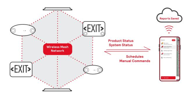
FirstLink is a standalone wireless system which integrates all necessary emergency lighting components with an app installed on a tablet or smartphone.
